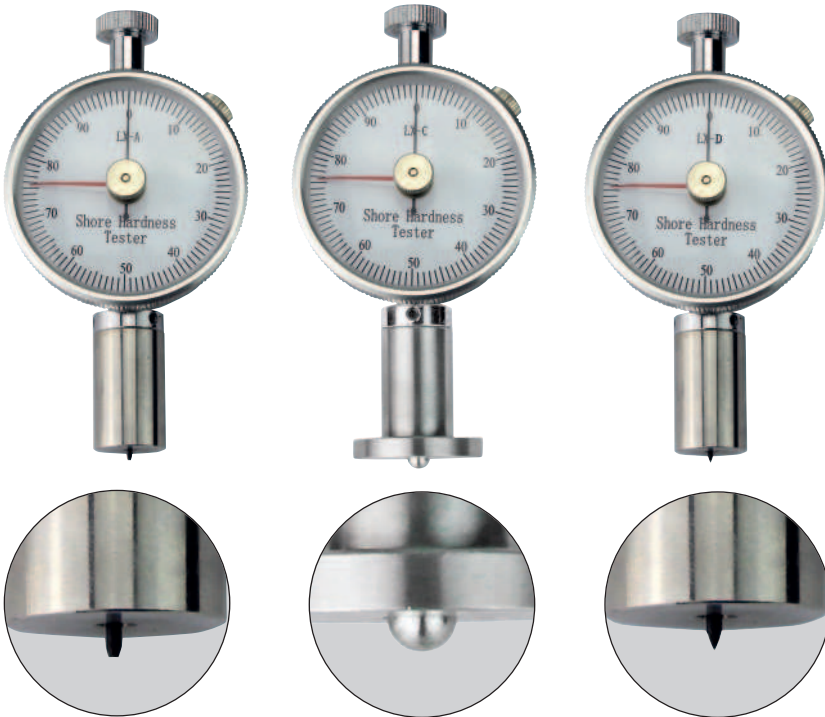
A: Flache Kegelspitze (ø 0,79 mm), 35° Flat cone point, (ø 0.79 mm), 35° C: Kugel 2,5 mm Spherical 2.5 mm D: Kegel, 30°, SR 0,1mm Sharp cone point, 30°, SR 0.1 mm
